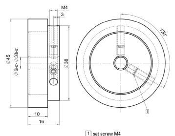
Recommended tolerance of the drive shaft diameter: g6
