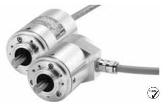
The Sendix 7053 Absolute Encoders – Singleturn offer Ex protection in a compact 70 mm seawater resistant housing, with an SSI interface and optical sensor technology.
