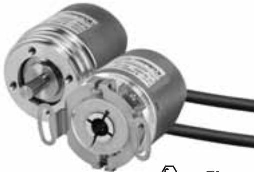
The Sendix F36 multiturn with the patented Intelligent Scan Technology™ is an optical multiturn encoder in miniature format, without gears and with 100% insensitivity to magnetic fields. With a size of just 36 x 42 mm it offers a through hollow shaft of up to 8 mm or a blind hollow shaft of up to 10 mm.
